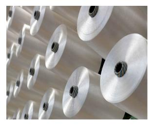
Rayon is also called Artificial Silk, which is a manufactured regenerated cellulose fiber, it is made from purified cellulose, primarily from wood pulp or cotton pulp.
